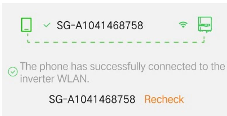
6. Tap "Next" at the lower part of the screen to connect the inverter to the home network. Select the home network WLAN and enter the password. The symbol "✓" indicates a successful connection to the home network WLAN.
