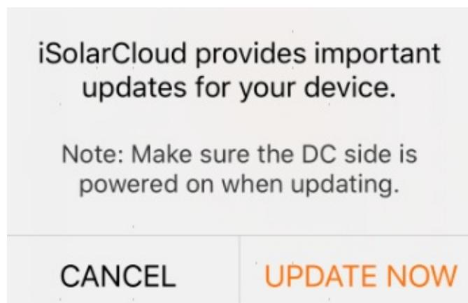
11. Tap "UPDATE NOW" to prompt the phone to reconnect to the Internet. Disconnect the mobile phone from the inverter WLAN to ensure the phone can normally access the Internet. Then connect the mobile phone to the local network, or enable the "Mobile data".
